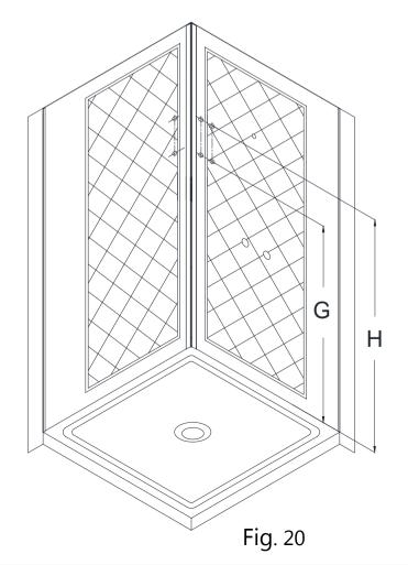
18. Mark the location for the **Shelf brackets (04)** according to the measurements in <u>Fig. 20</u> and <u>Fig. 21.1</u>.
