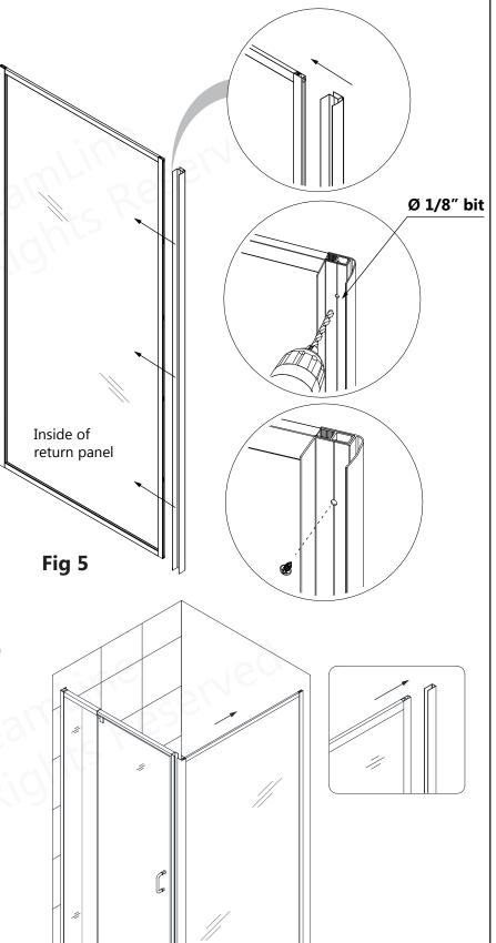
6. Slide the Return Panel Assembly (#09) into the Return Panel Wall Profile (#11). (Fig 6)
