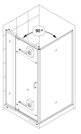
**9.** From inside the shower, drill holes into the top and bottom Expanding rails through the predrilled holes using an Ø 1/8" drill bit.
