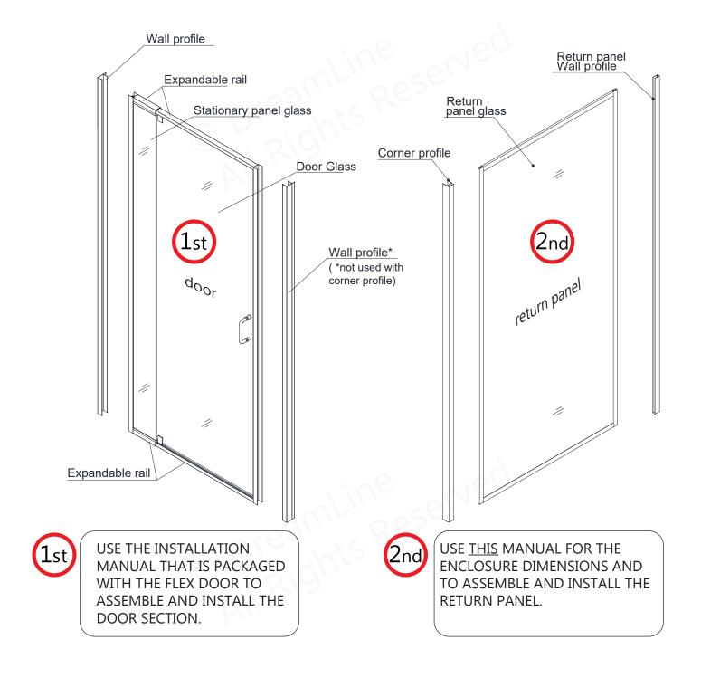
**NOTE:** This model is reversible for left or right-hand installation. This manual will show the right-hand return panel installation. For a left-hand installation, simply begin on the opposite wall and reverse the orientation of the parts as necessary.
