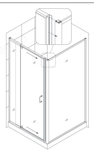
**8.** Make sure the **Door assembly (#02)** is fully extended into the **Wall profile (#01)** and the **Corner Profile (#10)**. Adjust top and bottom **Expanding rails** to the same length, making the door area square. Use a tape measure for accuracy.
