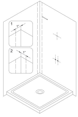
Measure the walls of the shower from the 1" (one inch) line in the corner (from Step. 1) to the points where you want Side panels (01) to end.
