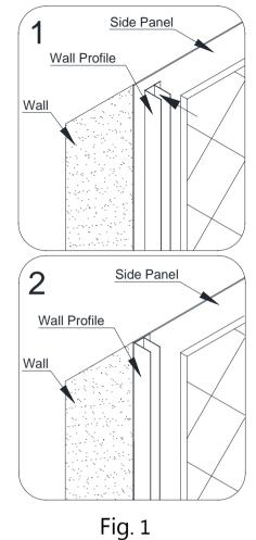
1. Place a mark on the walls with a distance of **1**" (**one inch**) from the corner and draw a plumb vertical line from top to bottom.
